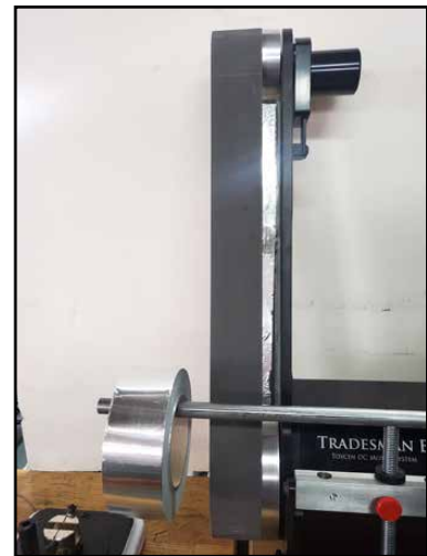
Use of foil tape to reduce static
